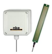
The operating principle is the measurement of voltage variation across the voltage divider bridge formed by the variable resistance probe (R = 300 kOhms dry, R = 2 kOhms wet) and the 0-10V analog input of the PRESS'O.
